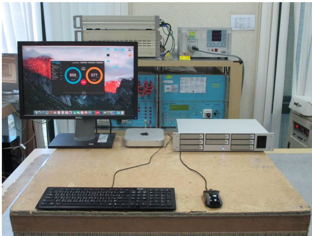
Set Up Photo of EFT
